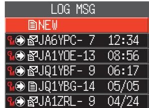
5. Rotate the **DIAL** knob to select to the message or image to be displayed, then press the **DIAL** knob.
